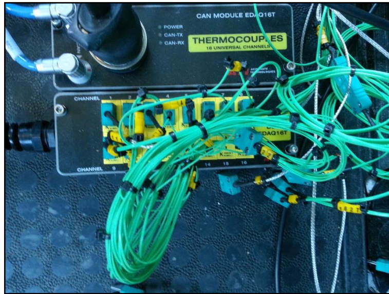
Figure 3.6. Illustration of the measurement setup for instrumentation channels
