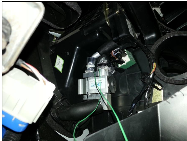
Figure 3.4. The instrumentation on the evaporator inlet and outlet
