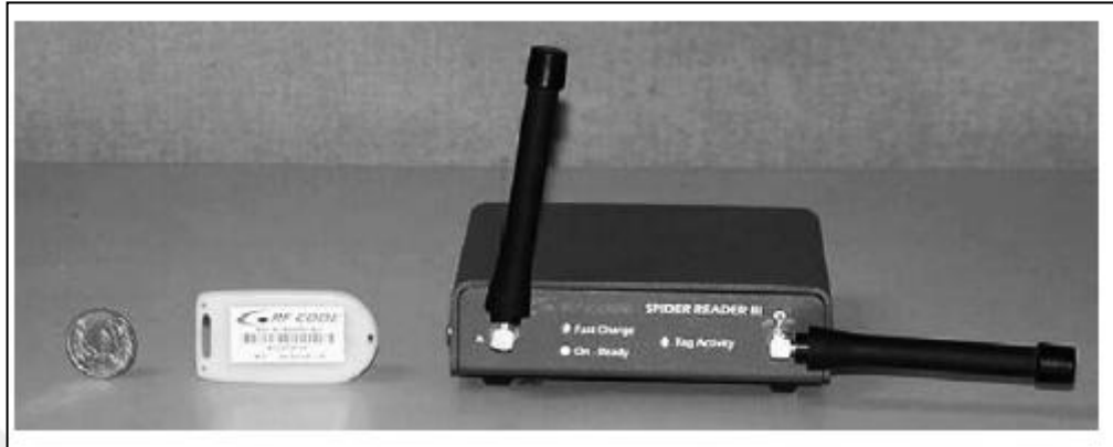
Figure 2.3. The RFID reader and tag used in prototype system [5]
