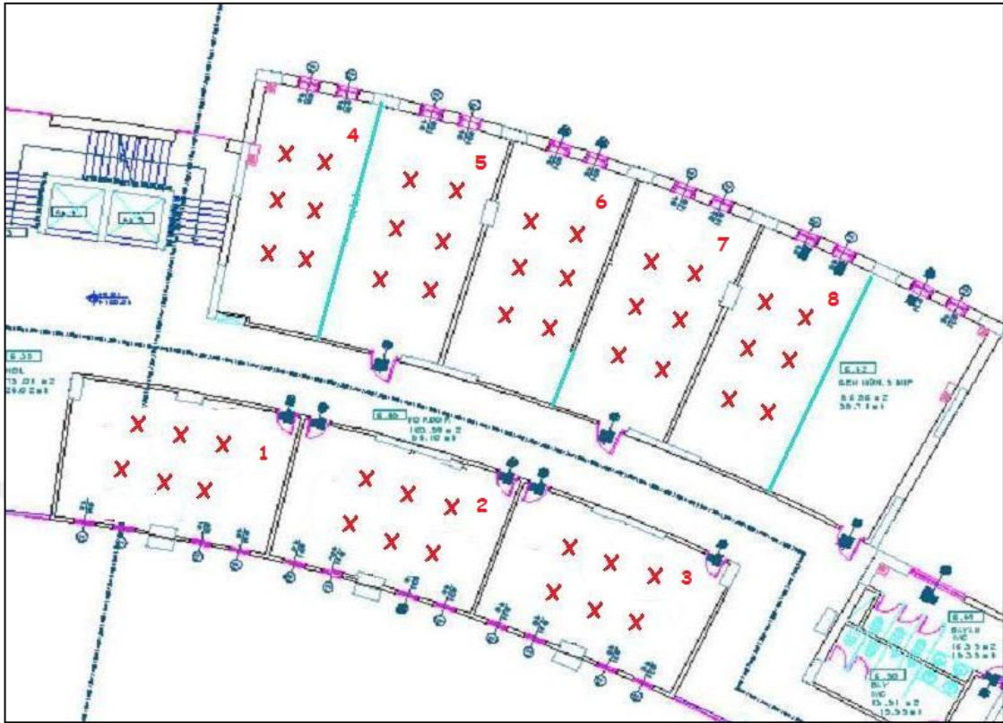
Figure 3.4. Floor plan of the test bed and RPs marked as red crosses
