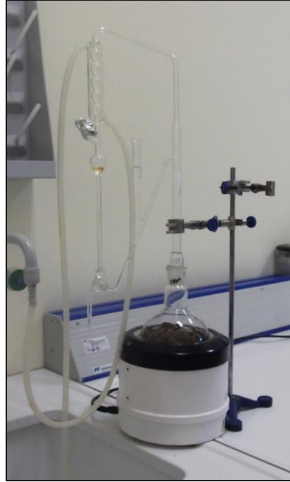
Figure 3.2. Essential oil extraction system composed of Clevenger apparatus and heater.
