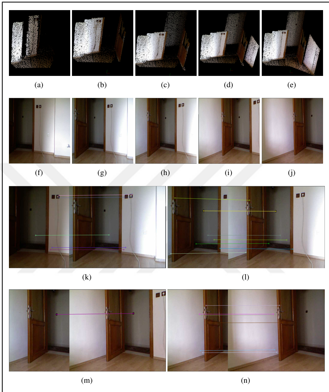
Figure A.4. Scene 4 images where (a)-(e) are 3D results, (f)-(j) are RGB images, (k)-(n) are matching visualization of the frames
