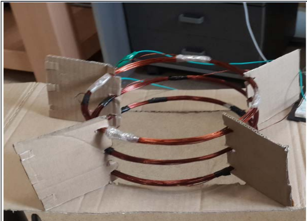
Figure 5.2. Constructed coaxial type coil with 15 turns
