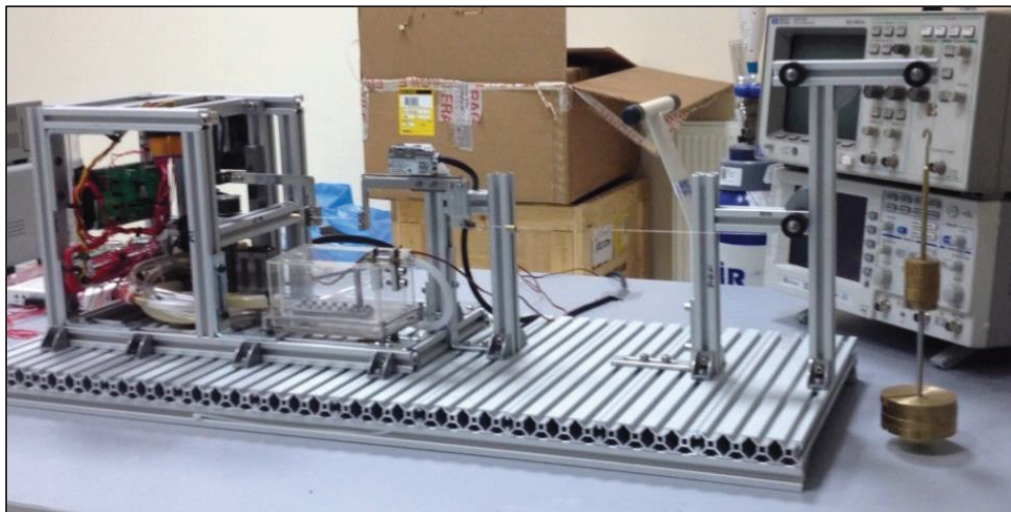
Figure 4.6 Experimental setup at isotonic test configuration
