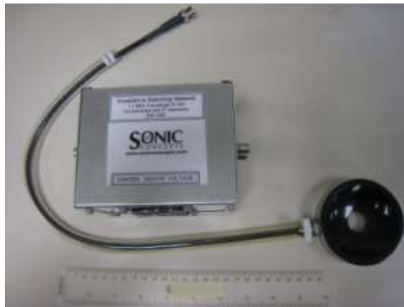
Figure 3.5. The H-102 transducer with impedance matching unit
