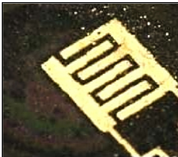
Figure 1. 15 Photograph of the fabricated porous silicon sensor
