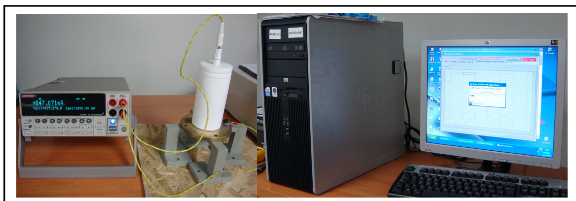
Figure 4. 1 Home-made computer controlled anodization and I-V measurement system
