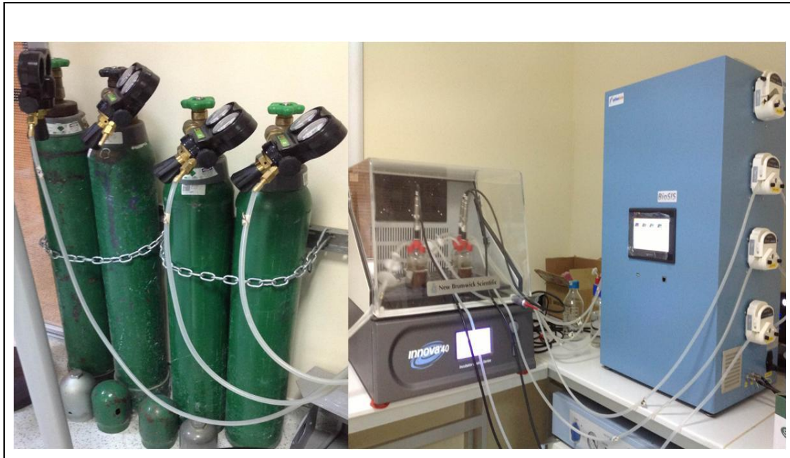
Figure 4.2. The bioreactor system used in the study. 100 % N_2 gas tanks each for each reactor vessels (left) and pH controller with pumps next to heating chamber including vessels (right).
