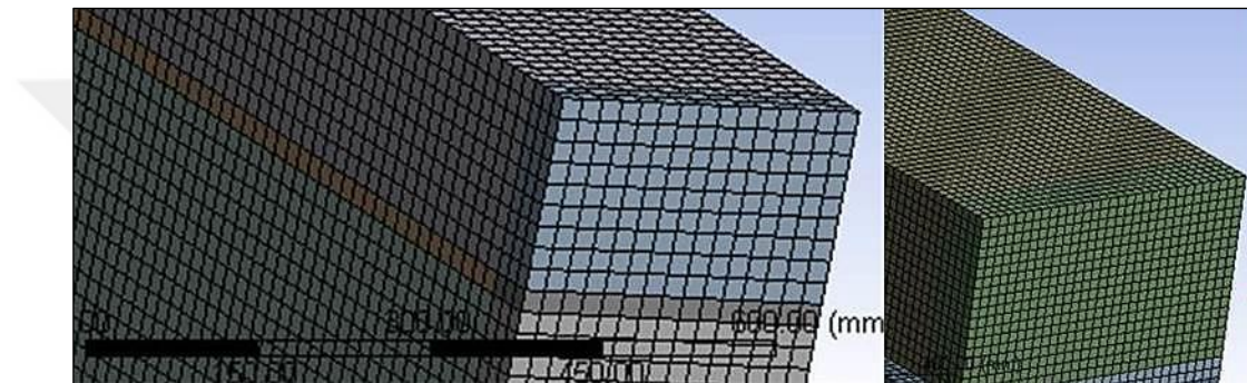
Figure 6.4. Mesh with wall distance of 17 mm for model A and 10 mm for model B
