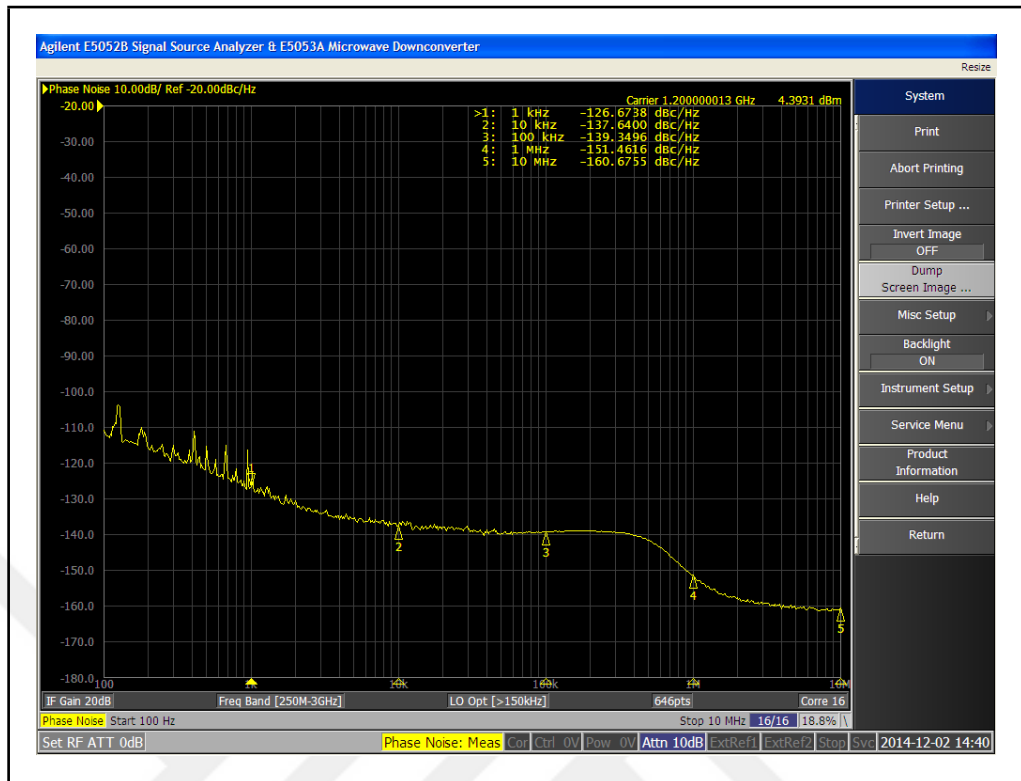
Figure 3.54: SSB phase noise measurement of combined SMA100A.
