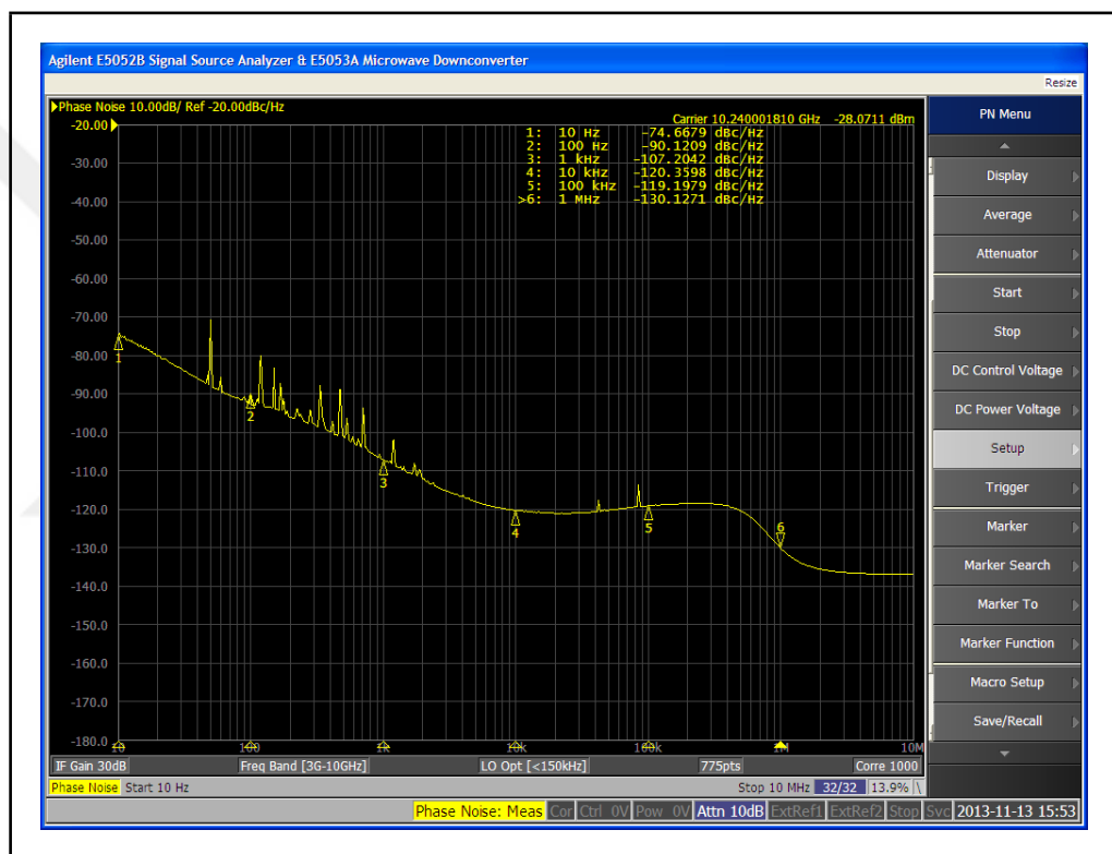
Figure 2.62: Agilent E5052B Signal Source Analyzer & SMA100 phase noise measurement
