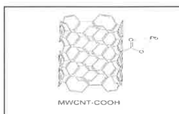
Figure 1.4. Multi-walled carbon nanotube-COOH (taken from Bulletin of the Korean Chemical Society (BKCS): Kinetic and Equilibrium Study of Lead (II) Removal by Functionalized Multiwalled Carbon Nanotubes with Isatin Derivative from Aqueous Solutions, 2013)
