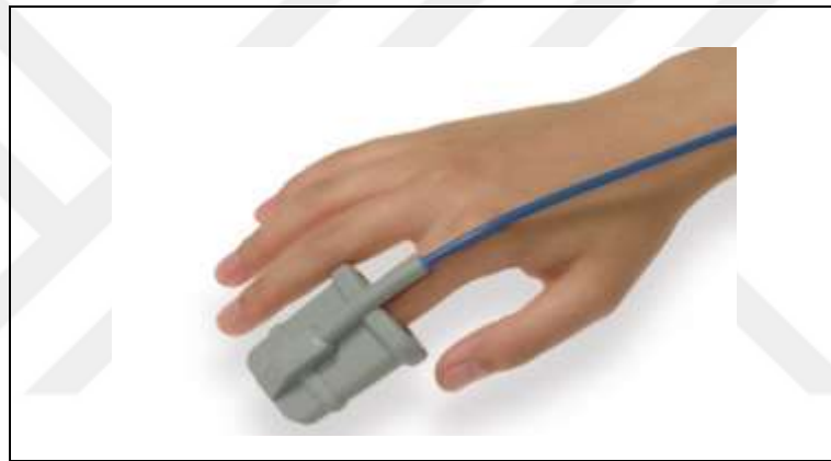
Figure 1.4. SpO 2 measurement from fingertip [18]
