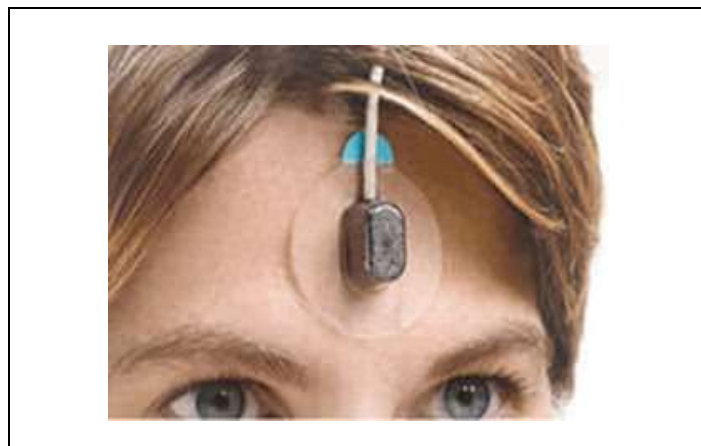
Figure 1.5. SpO 2 measurement from forehead [19]
