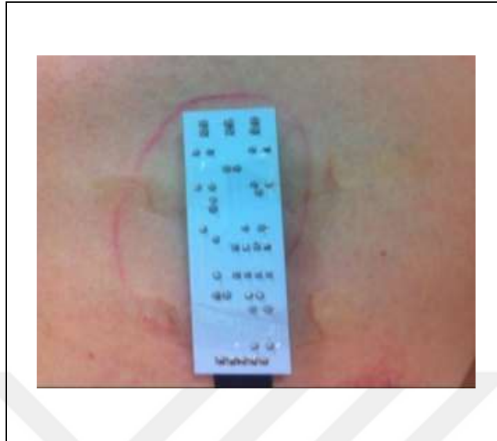
Figure 1.8. SpO 2 measurement from chest
