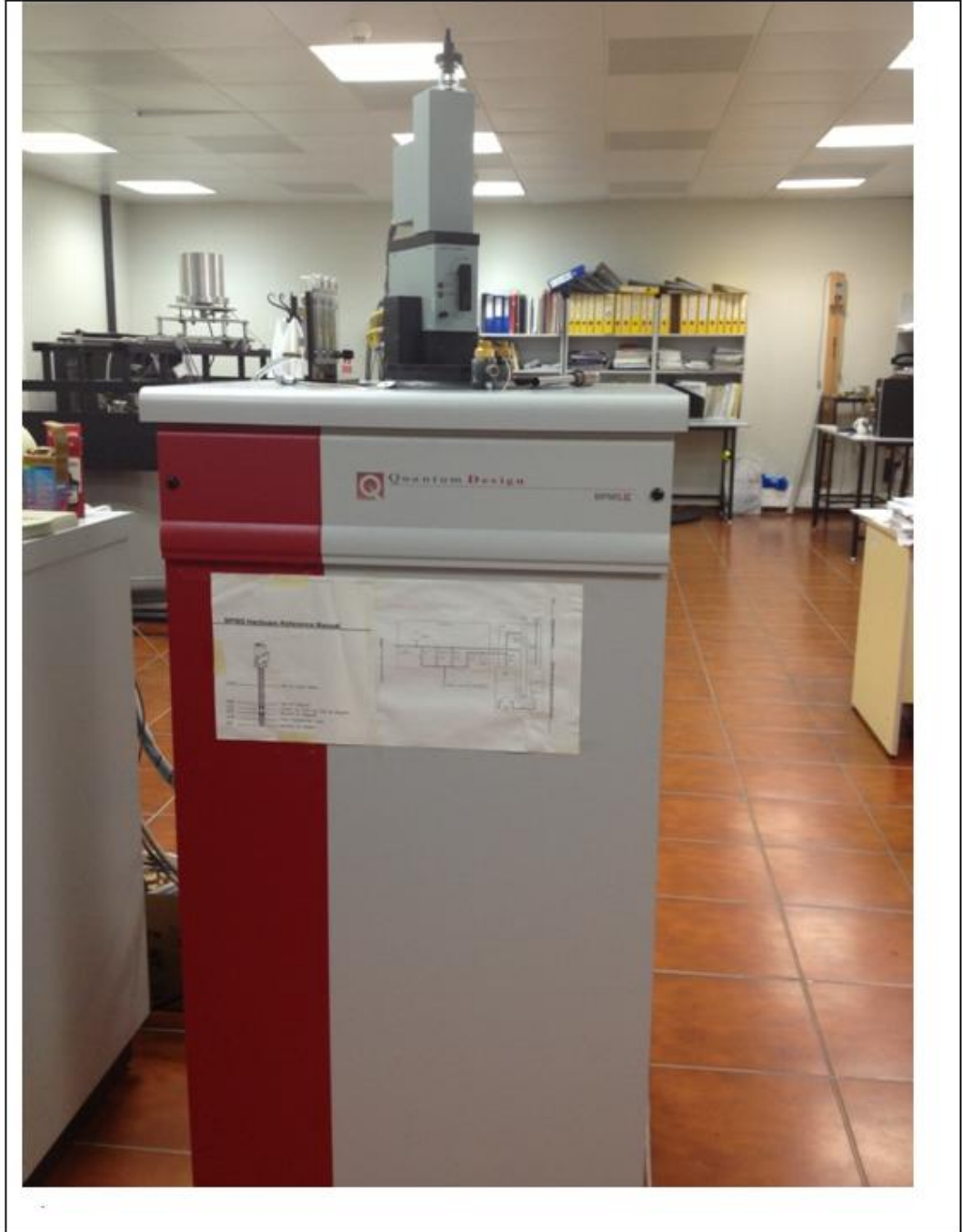
Figure C. 1 . MPMS-5 SQUID magnetometer from Quantum Design, Magnetic Laboratory at Tübitak-UME
