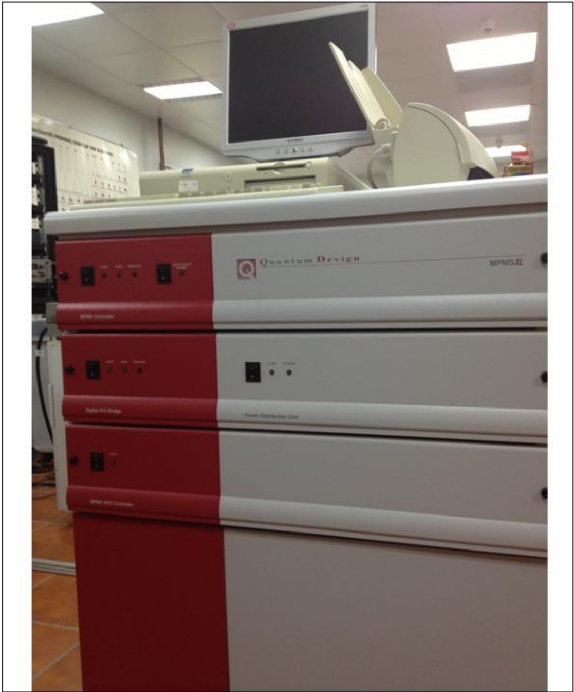
Figure C. 3. MPMS-5 SQUID magnetometer from Quantum Design, Magnetic Laboratory at Tübitak-UME.
