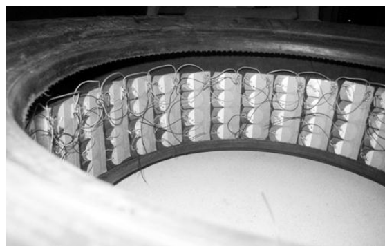
Figure 2.4. Piezo-ceramic bender elements in tire surface for generating electricity [25-27]
