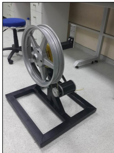
Figure 6.3. Structure where the DC motor and the Cam is placed
