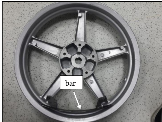
Figure 6.2. Cam obtained by placing a bar inside a circular part
