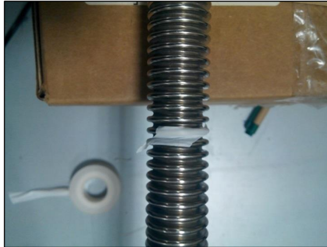
Figure 3.19. Coated tape on the pipe surface
