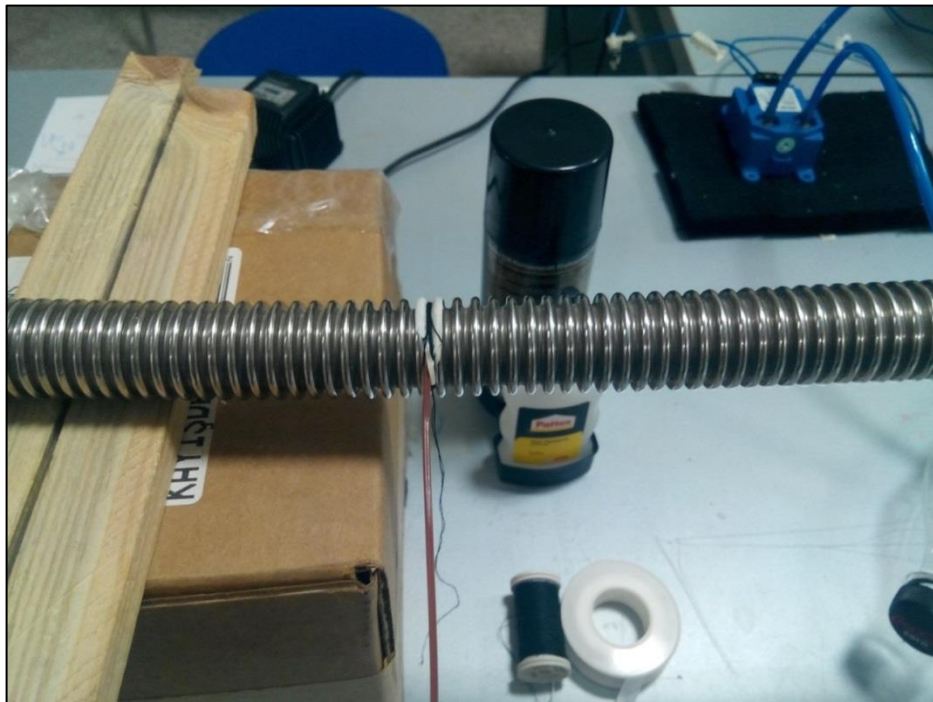
Figure 3.21. Thermocouple placed on the coated tape
