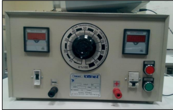
Figure 3.23. Transformer used in forced convection heat transfer tests
