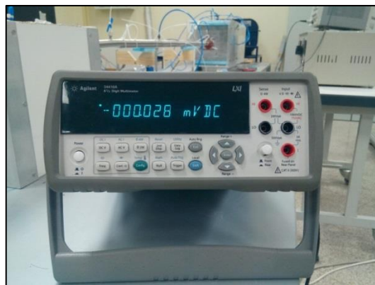
Figure 3.26. Multimeter used in pipe resistance tests
