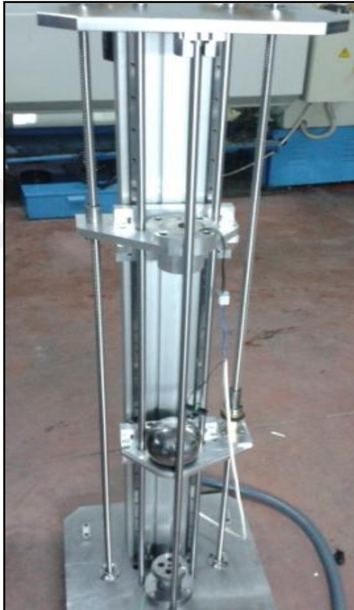
Figure 3.32. Assembling of the drop mass system
