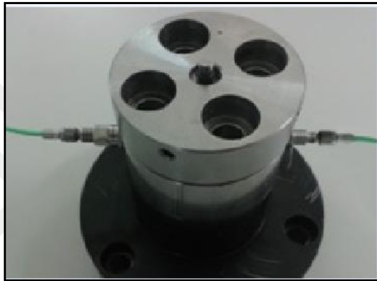
Figure 4.3. Oil filled closed chamber equipped with piston-cylinder unit, reference and test sensors
