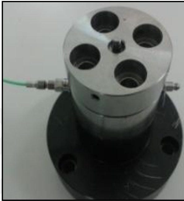
Figure 3.25. Mounted piston and quartz sensor
