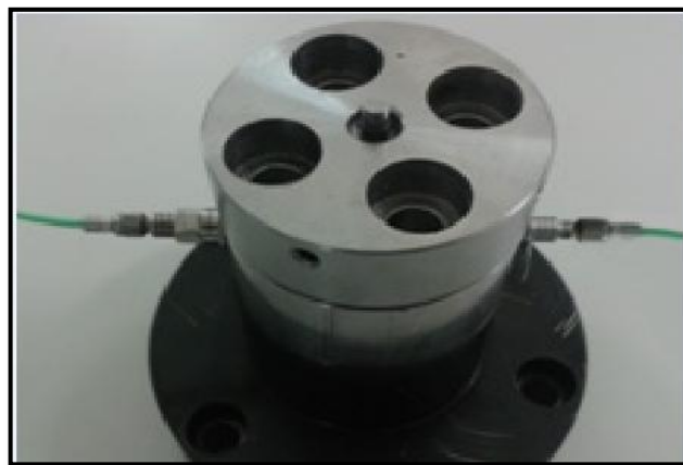
Figure 3.44. Oil filled closed chamber equipped with piston-cylinder unit, reference and test sensors
