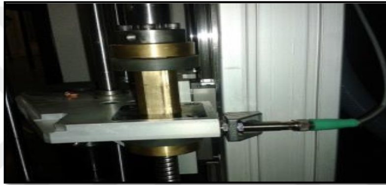
Figure 3.19. Lower reference position sensor for holder
