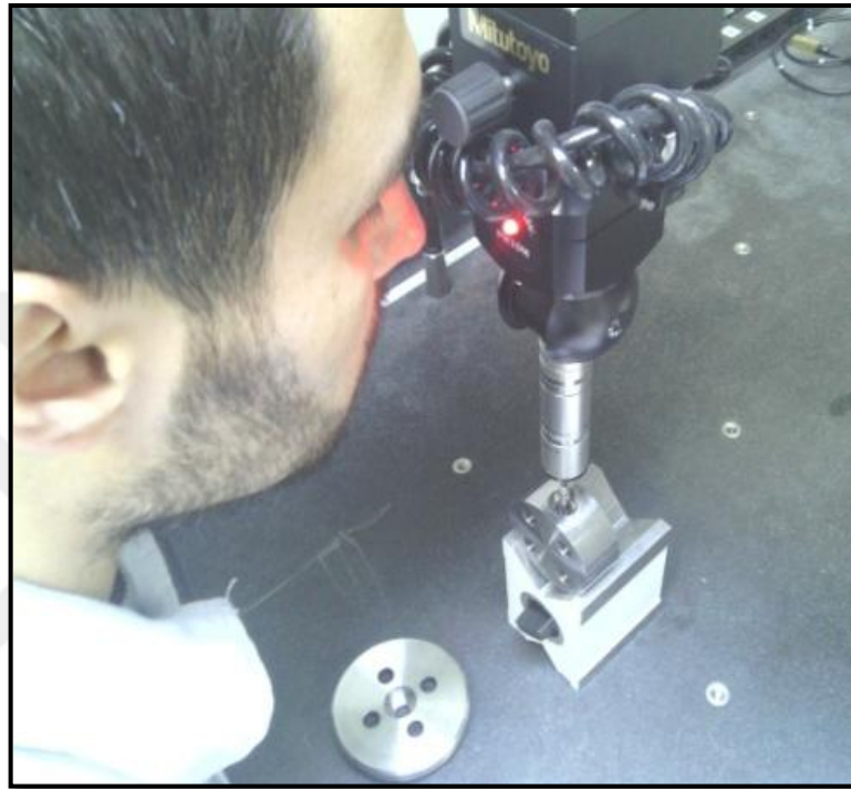
Figure 3.5. Dimensional Measurements of sensor hole-1
