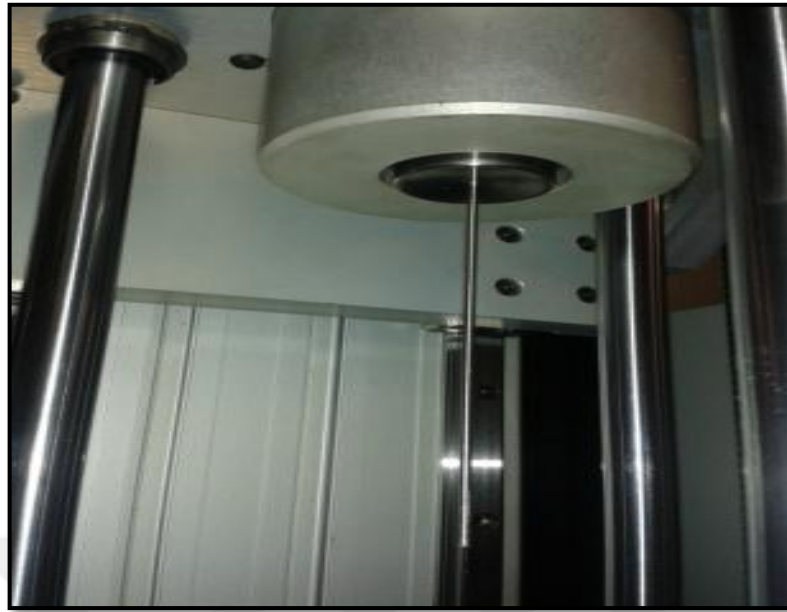
Figure 3.22. Concentric method for collision of sphere and piston-1
