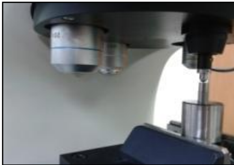
Figure 3.26. Piston hardness measurement setup
