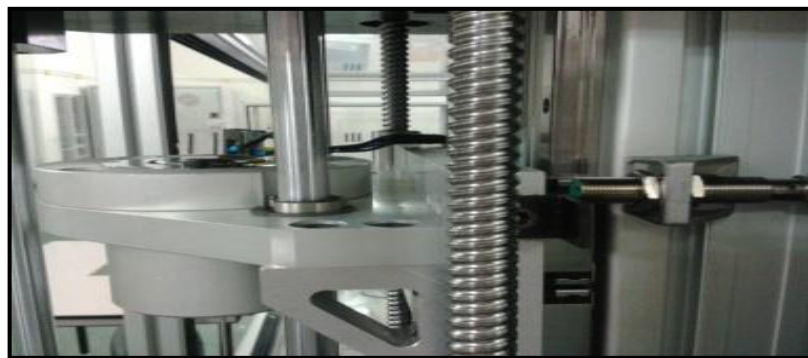
Figure 3.20. Upper reference position sensor for magnet
