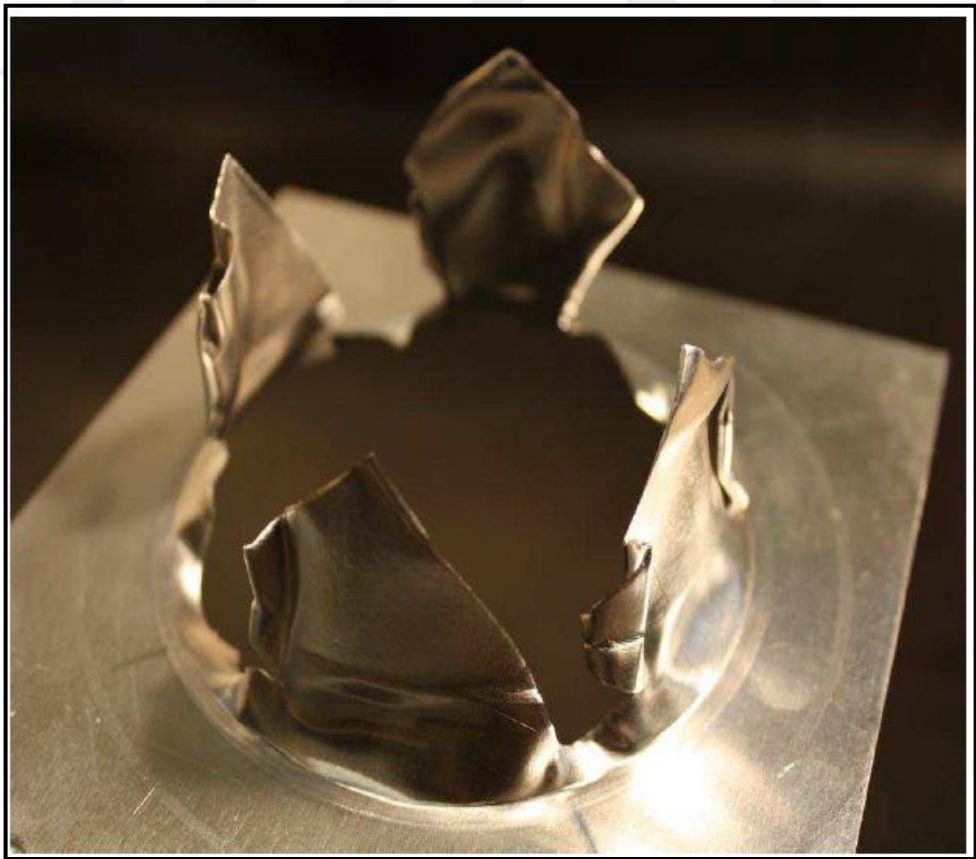
Figure 1.8. Burst aluminum diaphragm [47]
