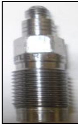
Figure 3.36. Dynamic pressure sensor up to 500 MPa
