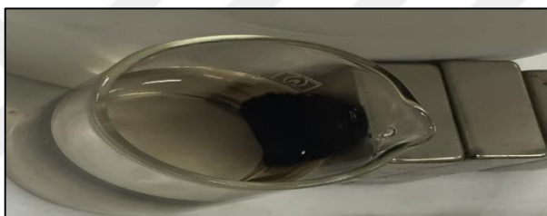
Figure 6.5. Magnet Separation of Magnetic Nanofluid
