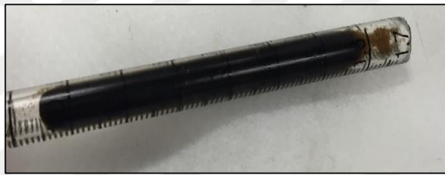
Figure 6.26. Captured magnetite-chitosan-TMZ nanofluid in the test section (0.5 %wt CD) after 1 hr
