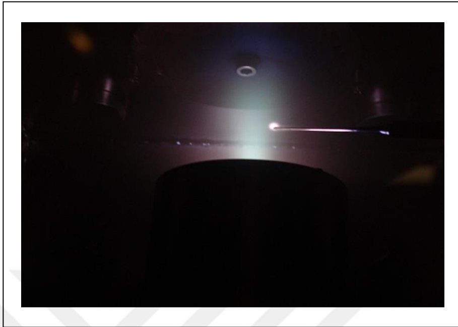
Figure 6.3. Langmuir probe in the plasma environment during sputtering process.
