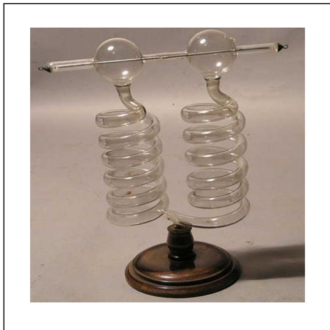
Figure 1.4. The figure of Hittorf tube [8]
