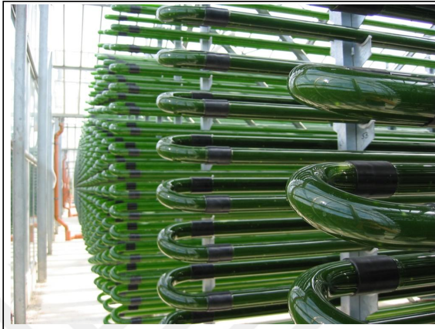
Figure 1.2. A closed-loop photobioreactor with glass piping. This design allows natural light to be absorbed by most of the culture. With these design and controlled parameters, algae cultures can be rapidly obtained. [21]
