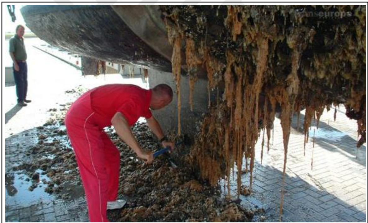
Figure 1.6. Biofouling as it is removed from a smaller vessel. This is a very good illustration of biofouling creating a rough surface that hinders the vessels ability to cruise smoothly. [42]
