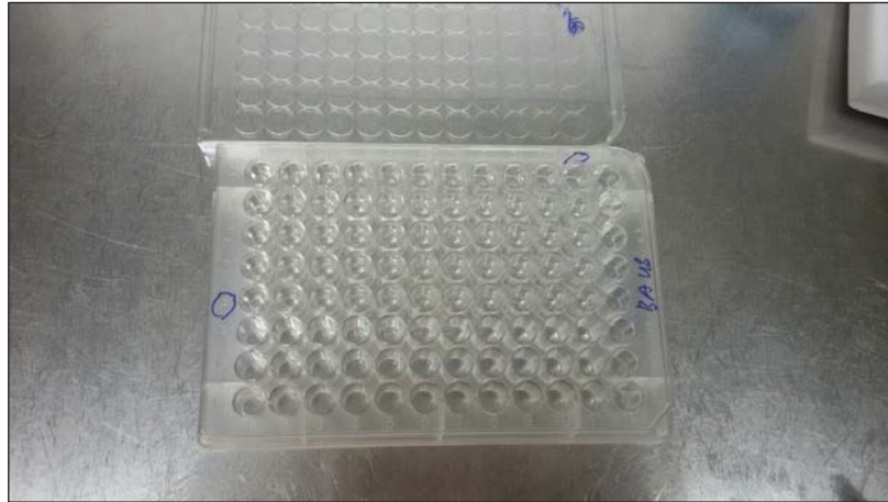
Figure 3.2. Adding methanol to fix the biofilm.
