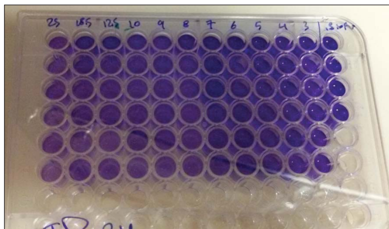
Figure 3.6. The re-solubilized liquid which measured at OD 595nm
