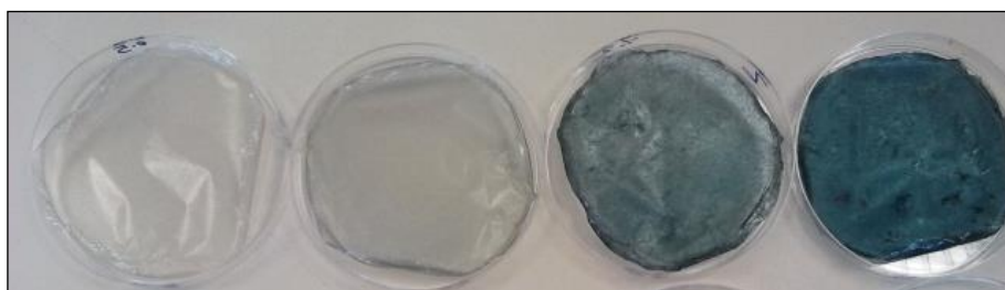
Figure 6.3. Hydrogel film samples with ratios of genipin/chitosan of Gnp05, Gnp1, Gnp2 and Gnp3, w/w from left to right
