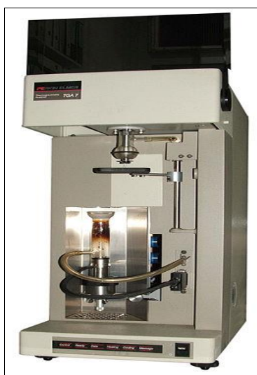
Figure 3.9. A typical TGA instrument [51].
