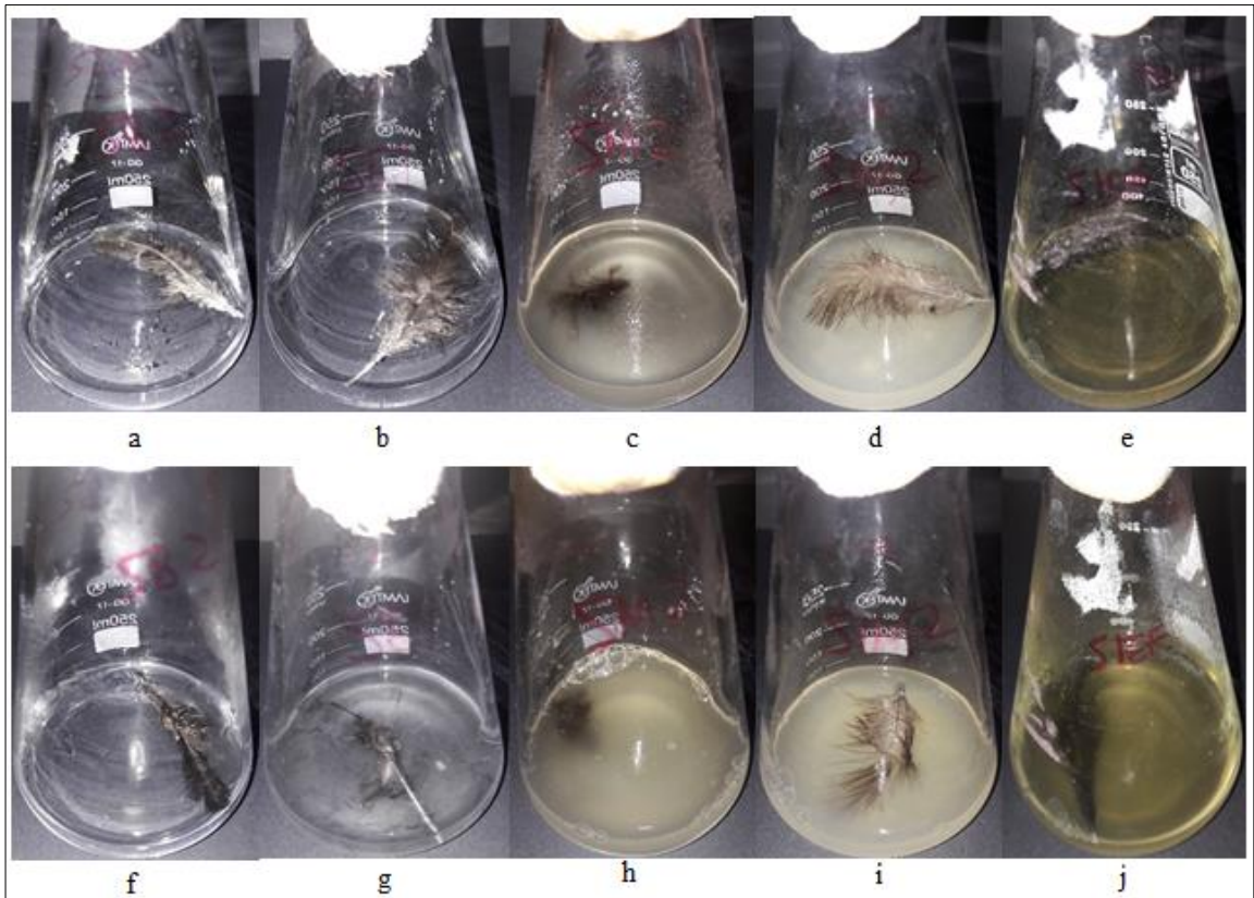
Figure 4.10. Whole feathers at 0 th hour inside, a) just water as negative blank b) 50 \mu L commercial protease as positive blank, c) non-induced Bacillus cereus d) feather-induced Bacillus cereus and e) supernatant of induced broth. Results after two days inside, a) just water as negative blank b) 50 \mu L commercial protease as positive blank, c) non-induced Bacillus cereus d) feather-induced Bacillus cereus and e) supernatant of induced broth. Erlenmeyers are swirled just once-a-day manually. Incubation temperature is at 37°C
