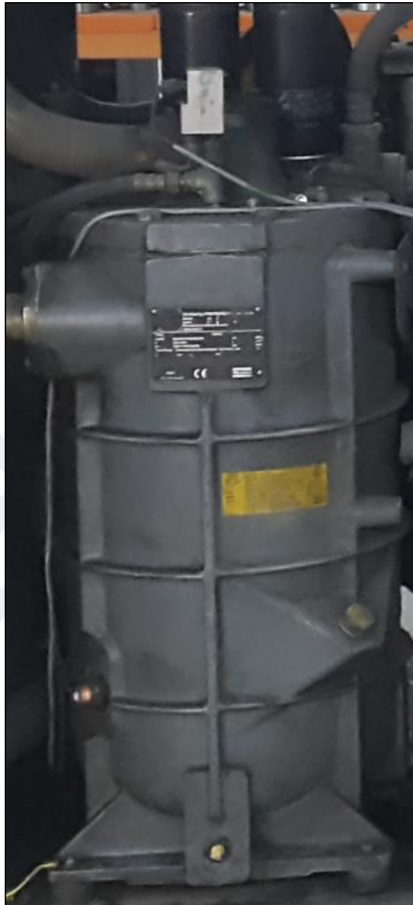
Figure 1.5. A vertical oil separation tank
