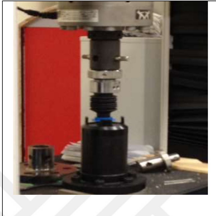
Figure 5.7. Bellow compression by using instron testing device
