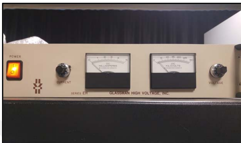
Figure 4.14. Picture of high dc voltage source.
