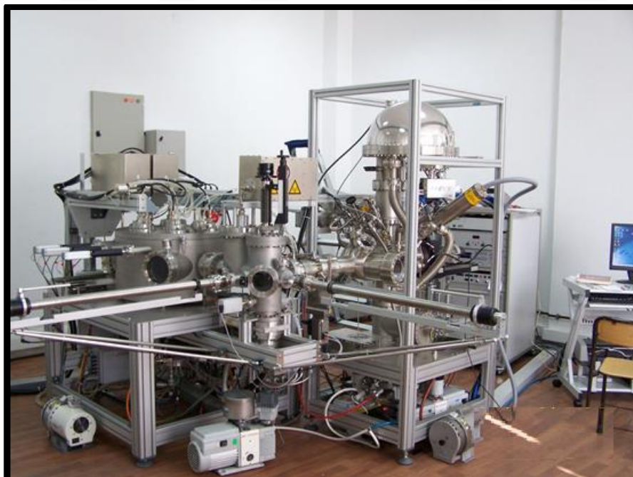
Figure 5.2. Cluster UHV chamber at Gebze Technical University for magnetron sputtering and surface characterization.
