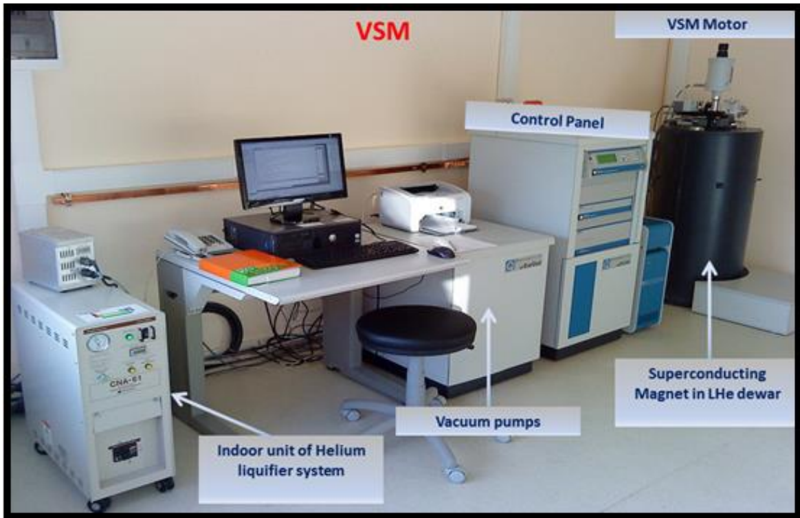
Figure 5.12. Quantum Design PPMS (9 T) System at Gebze Technical University for VSM measurements.
