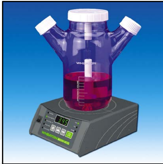
Figure 2.1. Representative image of MagnaFlask cell isolation apparatus on heater with magnetic stirrer.
