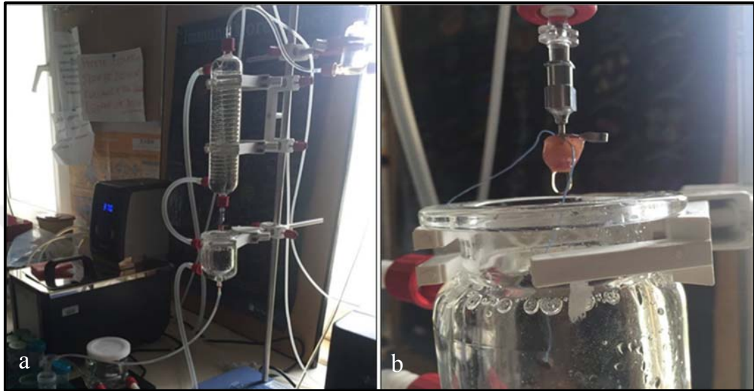
Figure A.1. Image of Langendorff Apparatus used for adult mouse heart digestion a) Complete picture of the Langendorff Apparatus b) Heart sample was cut and the tip of the apparatus inserted into the aorta for successful digestion.
