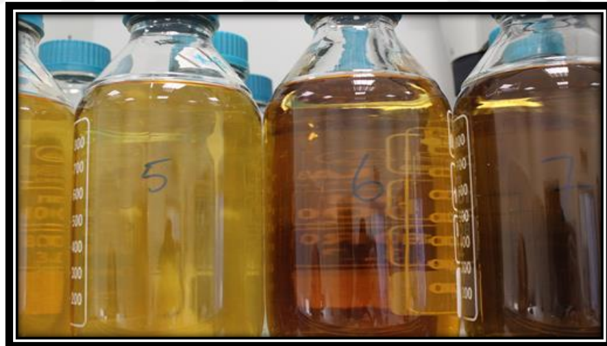
Figure 3.12. Samples of microorganism + phosphorus phosphorus (BM + PA + PP + AB + ML + BC + AN + Phosphorus) fertilizer kept at 25 ° C temperature and 60% humidity
