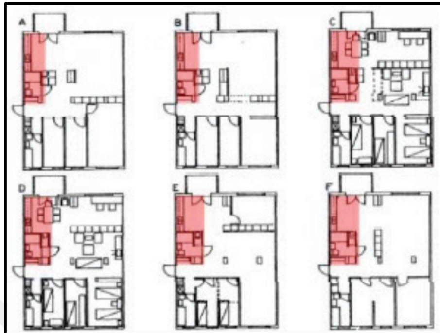
Figure 4.9. Van Der Rohe's Weissenhof Project, configuration of other spaces suitable for different uses by keeping wet volumes stable [2].
