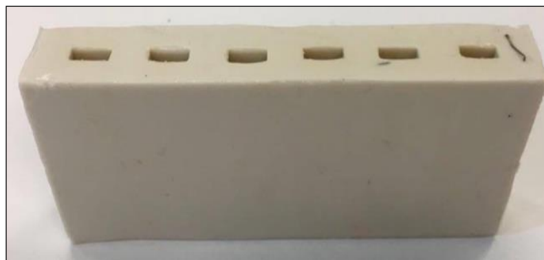
Figure 4.4. Silicon mold used for curing the resins.
