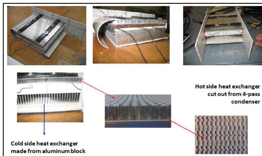
Figure 2.15. Thermoelectric system prototype for CTS
