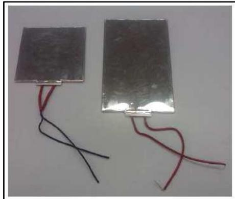
Figure 3.15. Plate type heaters
