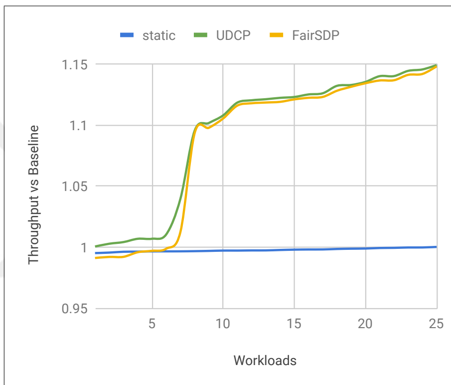
Figure 5.7. Results over 25 workloads on an 8-threaded system
