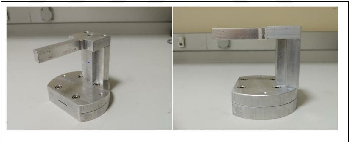
Figure 6.10. Image of the manufactured version of the beam holder designed for the model
