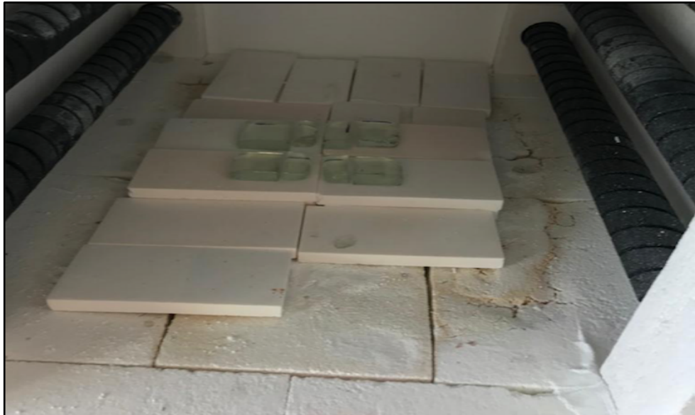
Figure 3.3. Image of production process of glass-ceramics in the furnace
