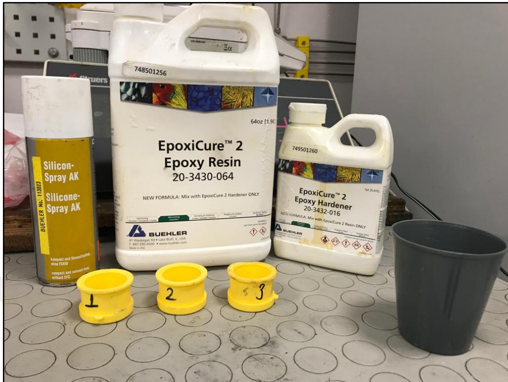
Figure 3.18. Materials used in preparing cold bakelite process
