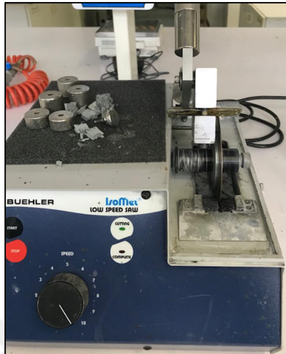
Figure 2.11. Cutting of produced glass samples with BUEHLER IsoMet Low Speed Raw device
