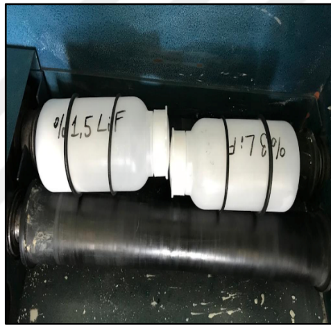
Figure 2.7. Performing the homogenization process in the ball mill
