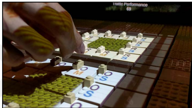
Figure 4.6. Users can change the land use pattern by adding, reducing and modifying optically labeled Lego bricks [7].
