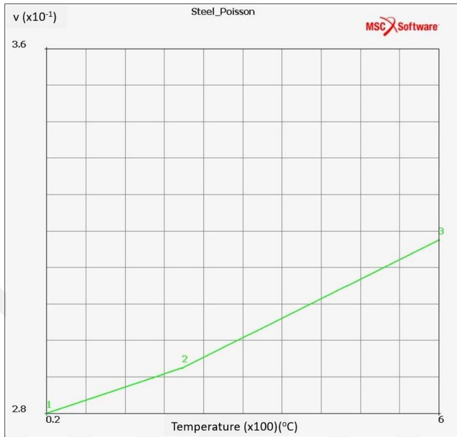
Figure 3.6. Temperature dependent Poisson's ratio of steel.
