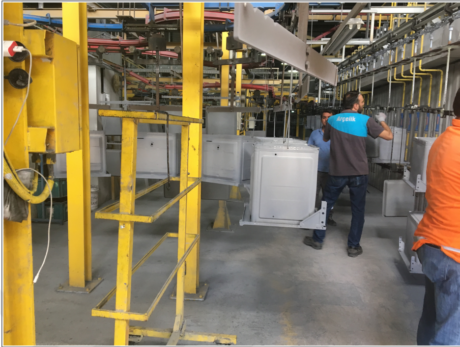
Figure 3.13. Glass frit coated oven cavities on production line.
