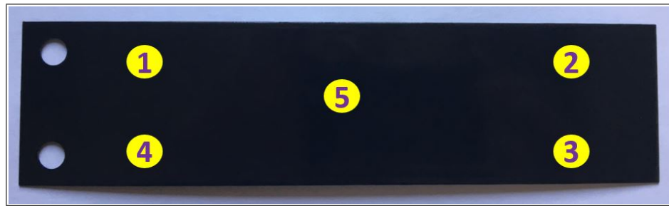
Figure 3.10. Glass film thickness measurement points on specimen.
