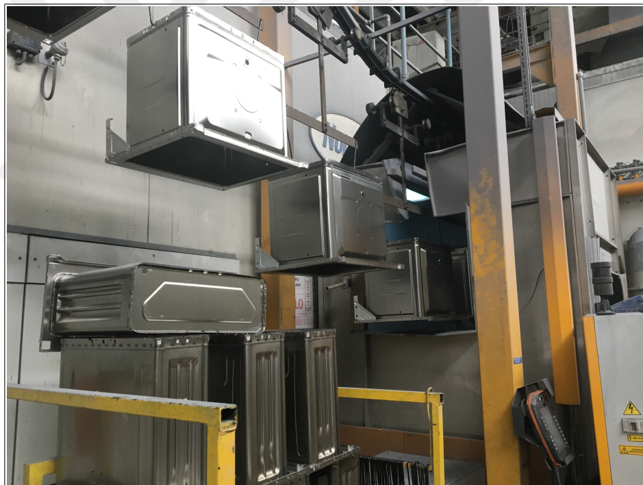
Figure 3.12. Uncoated oven cavities on production line.
