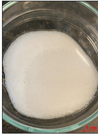
Figure 2.1. Micro bubbles with 200 \mu\text{l} / min flow rates and 0.6, bar gas pressure collected in a small glass container produced.
