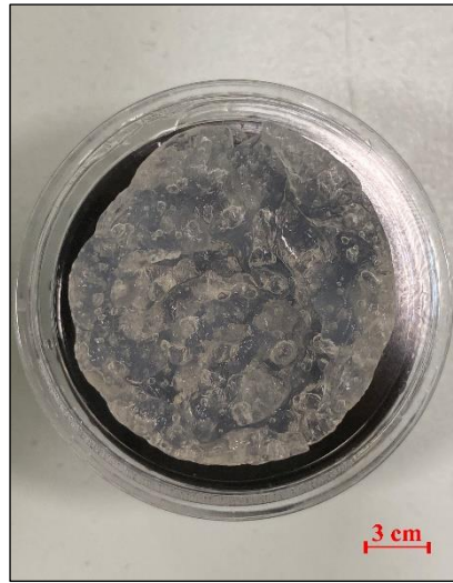
Figure 2.2. Porous hydrogel structure containing Hypericum perforatum and honey active ingredients produced in the experimental work.
