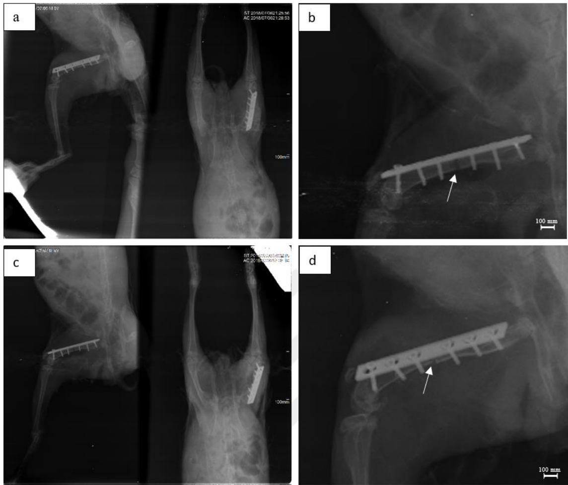
Figure 3.2. X-ray evaluation after implantation (at day 1) for TiN/(TiMg) N plates. (a, b) TiN and, (c, d) (Ti, Mg) N thin film coated plates.
