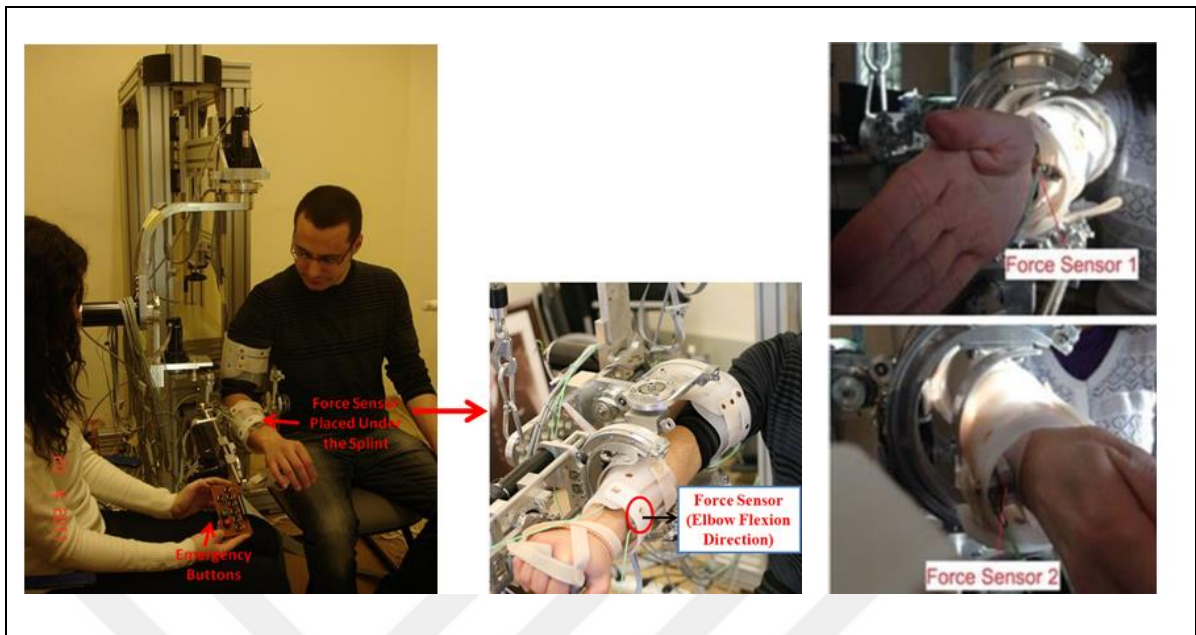
Figure 3.4. Arm splint and force sensors of RehabRoby
