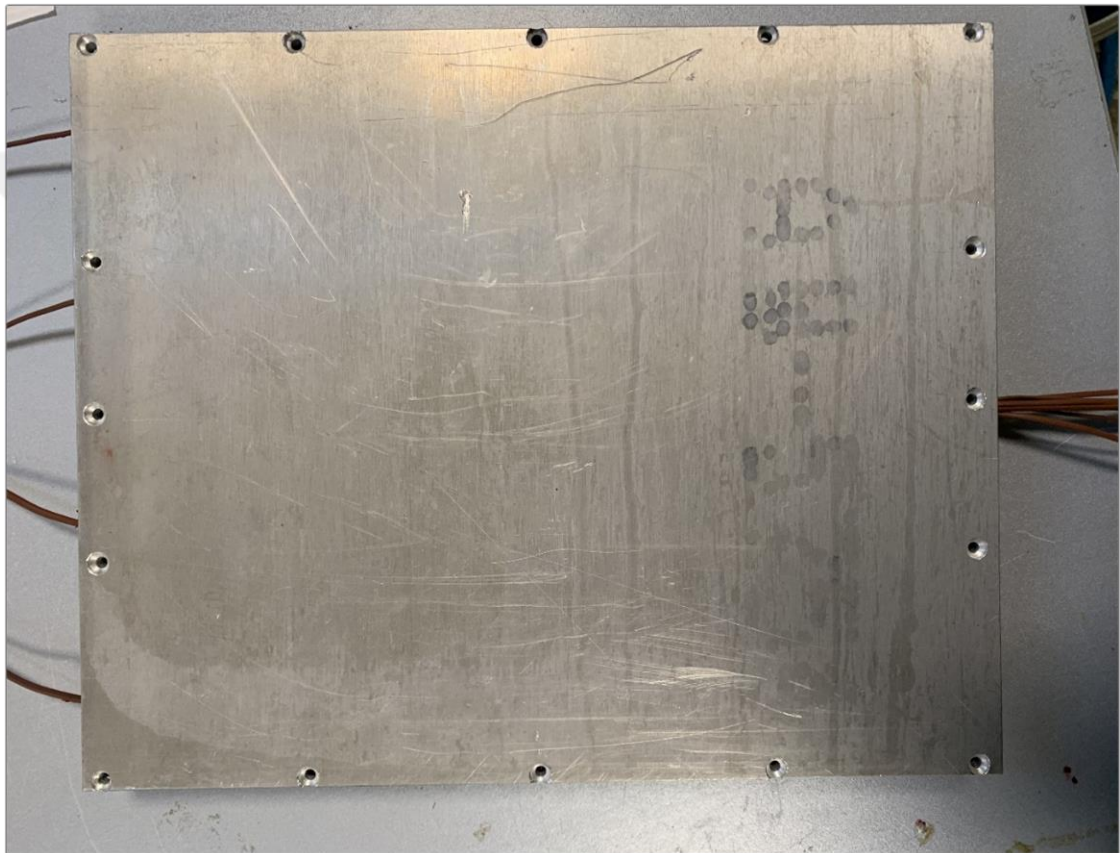
Figure 5.3. Top view of the plate condenser made of aluminum
