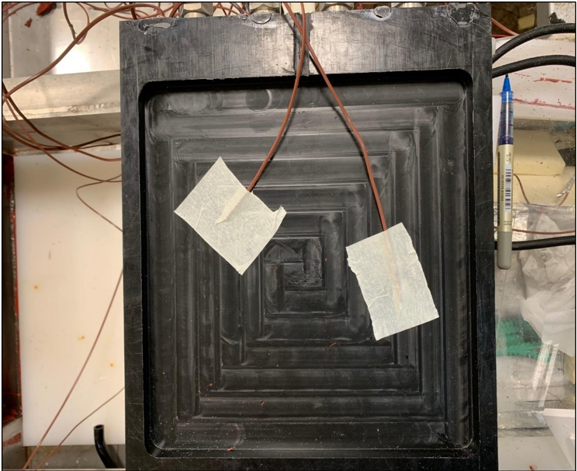
Figure 5.6. Thermocouple placement under the bottom part
