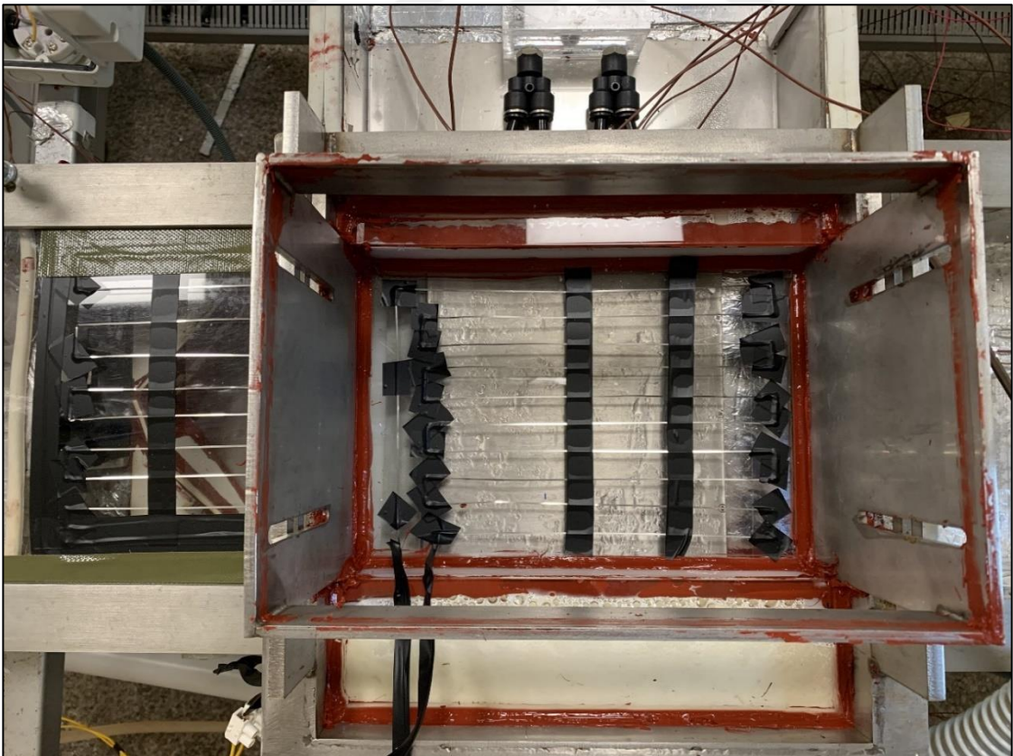
Figure 5.17. Complete view of the plate condenser test section
