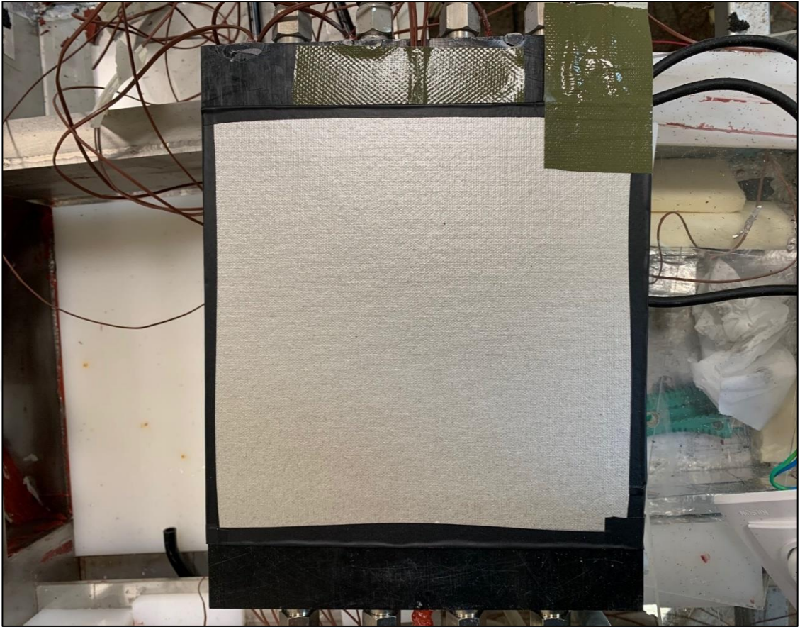
Figure 5.8. Resistance heater placed under the polyamide base.
