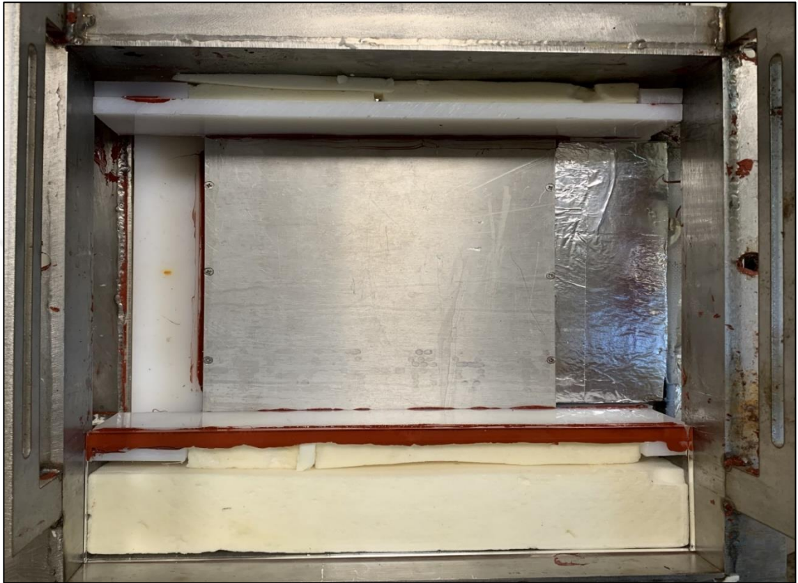
Figure 5.15. Plate condenser placement inside the test section
