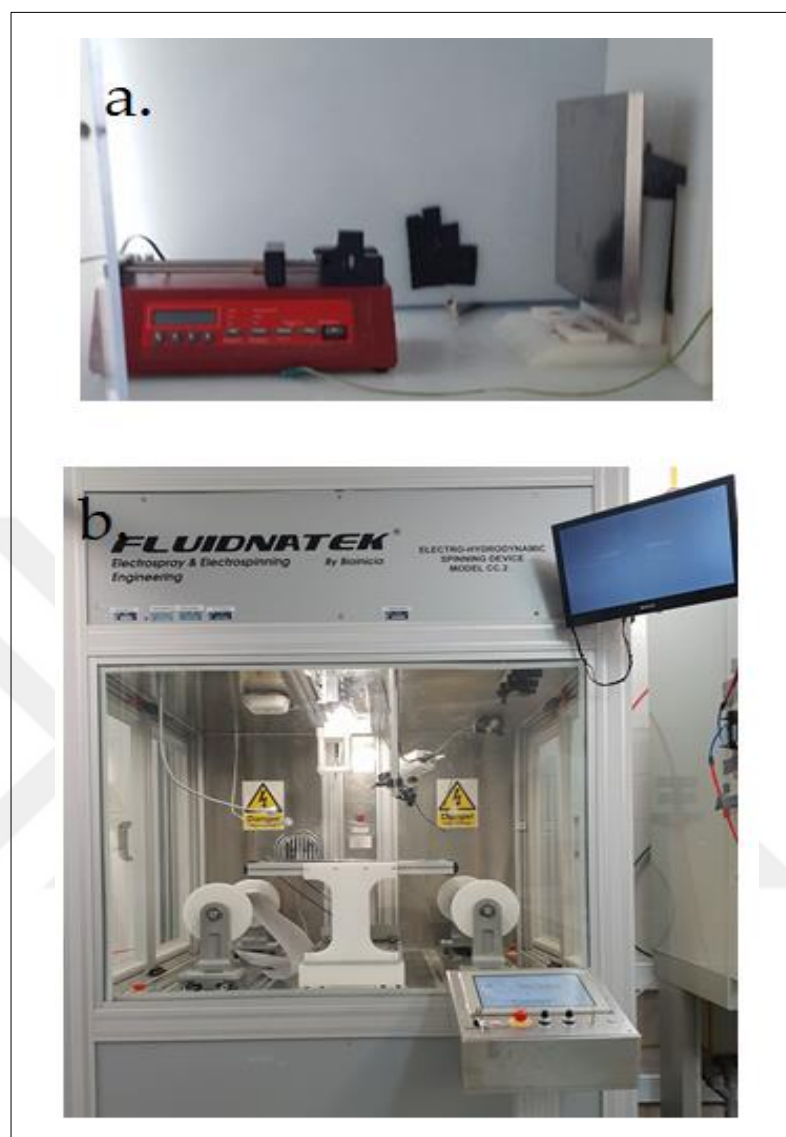
Figure 2.2. The (a) first and (b) second electrospinning systems.
