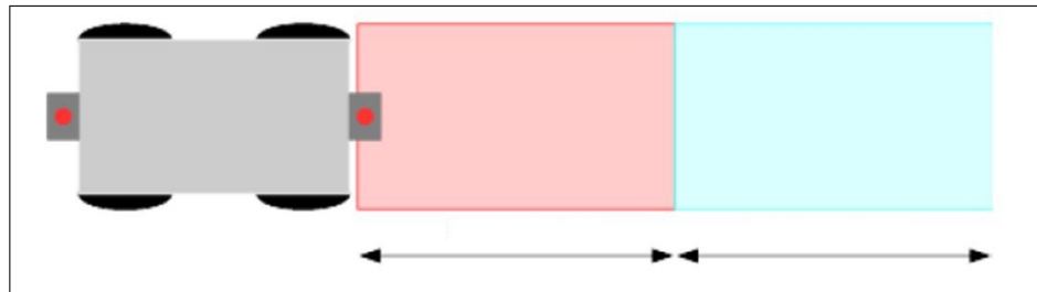
Figure 3.6. Breaking areas of the robot on follow mode
