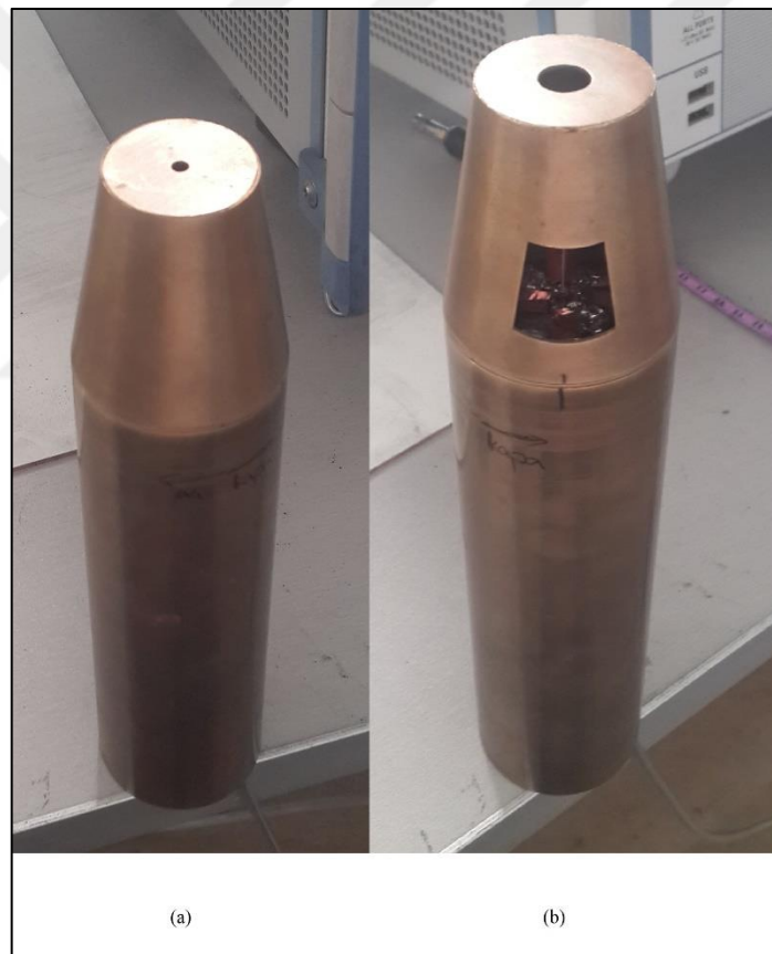
Figure 4.3. Bulkhead configurations. (a) Side view of windowless configuration, (b) Side view of windowed configuration
