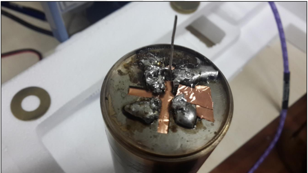
Figure 4.1. 3 cm monopole antenna soldered on mock missile.
