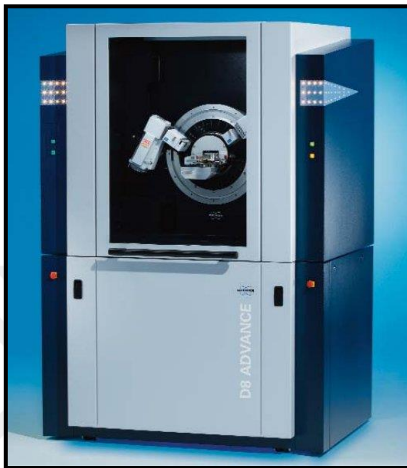
Figure 2.7. The X-Ray Diffractometer D8 ADVANCE [65].
