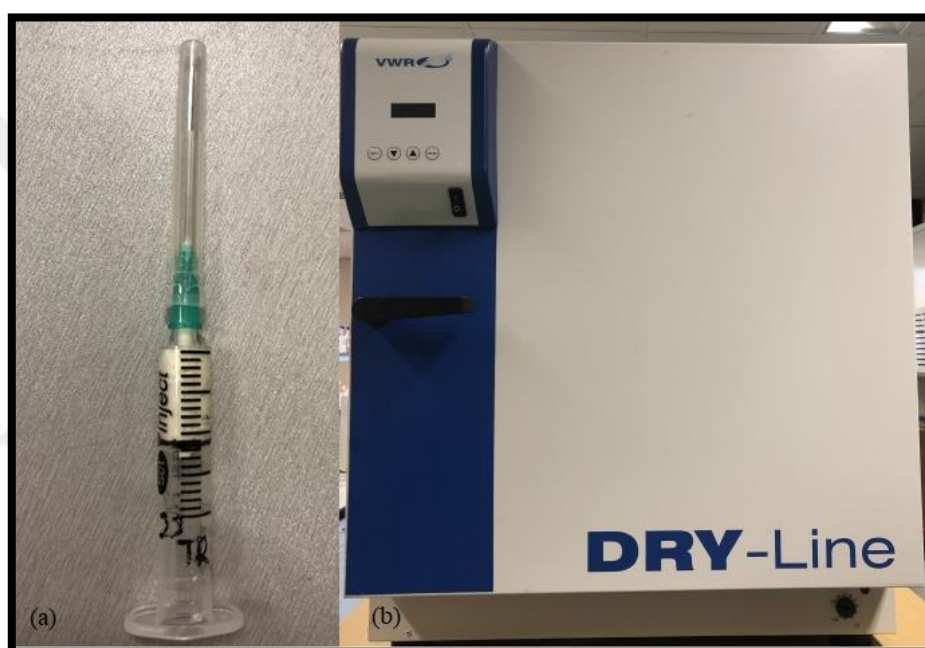
Figure 2.4. (a) Cement placed in syringe (b) before the incubation step.
