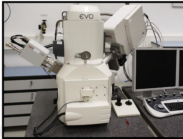
Figure 2.8. The Carl Zeiss EVO 40 scanning electron microscope.
