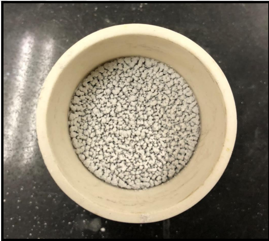
Figure 2.2. Synthesized TTCP powder
