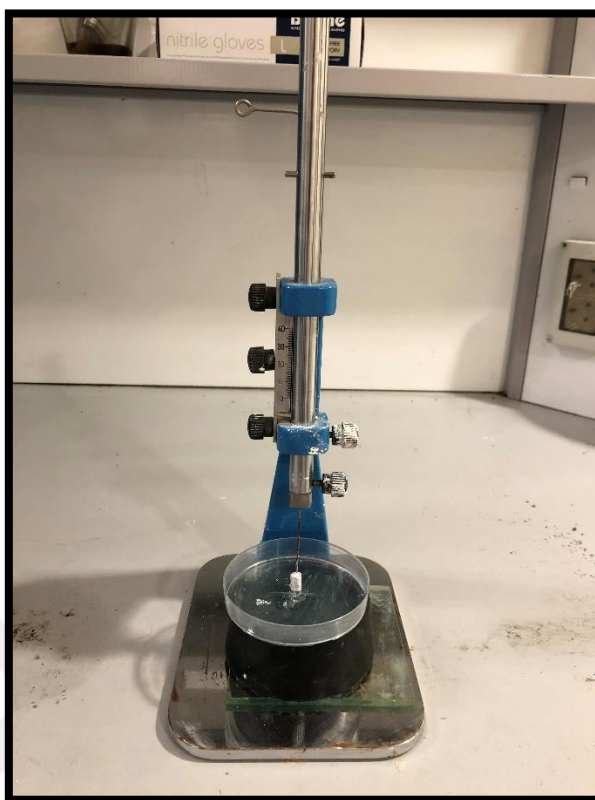
Figure 2.10. The Vicat apparatus for the setting time assesment.
