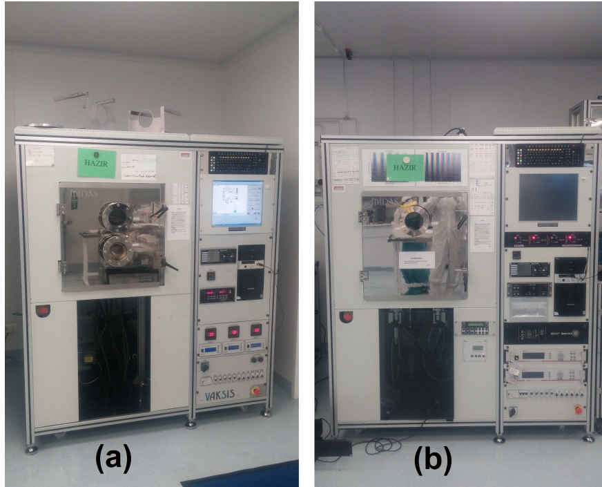
Figure 3.3: VAKSIS (a) thermal evaporator and (b) sputtering systems.
