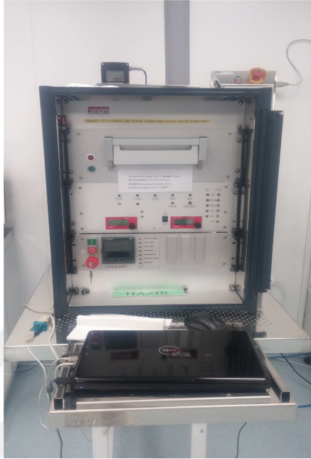
Figure 3.7: ATV Technologie GmbH, SRO-704 RTA system.
