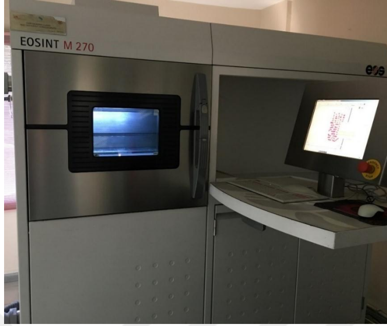
Resim 3.10: Lazer sinter cihazı (EOS GmbH Electro Optical Systems)
