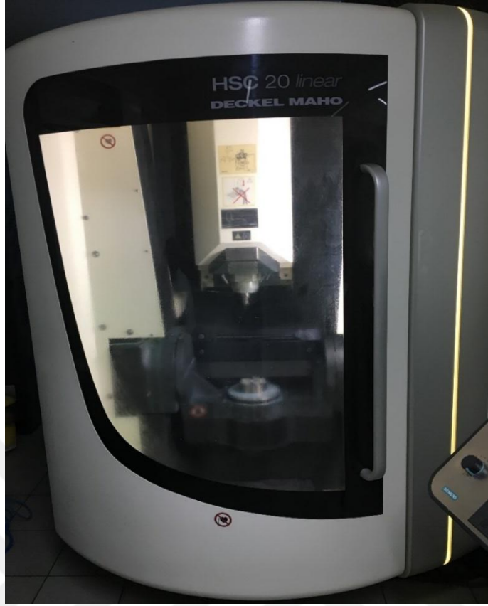
Resim 3.13: CAD/CAM Milleme makinesi (DMG / HSC 20 Linear Deckel Maho)
