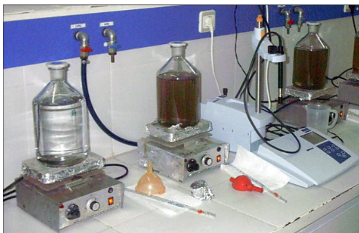
Figure 5.4. Experimental set-up of batch experiments with TCE
