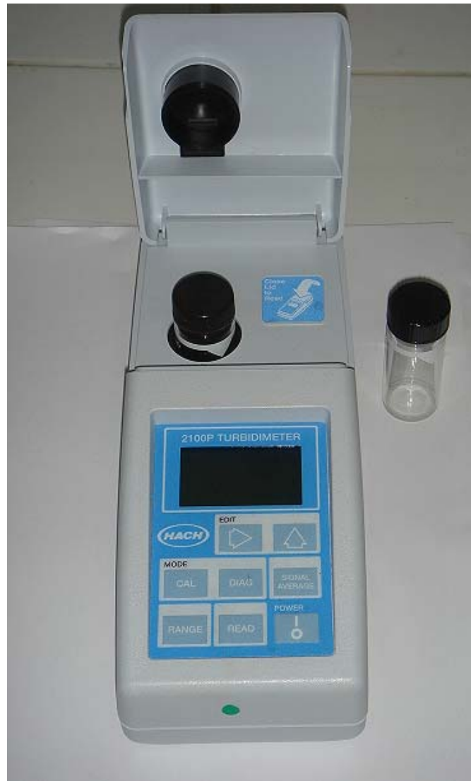
Figure 3.3. HACH 2100P Turbidimeter used in the experiments
