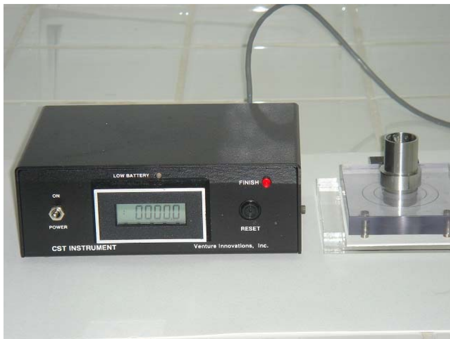
Figure 3.2. Capillary suction time (CST) apparatus
