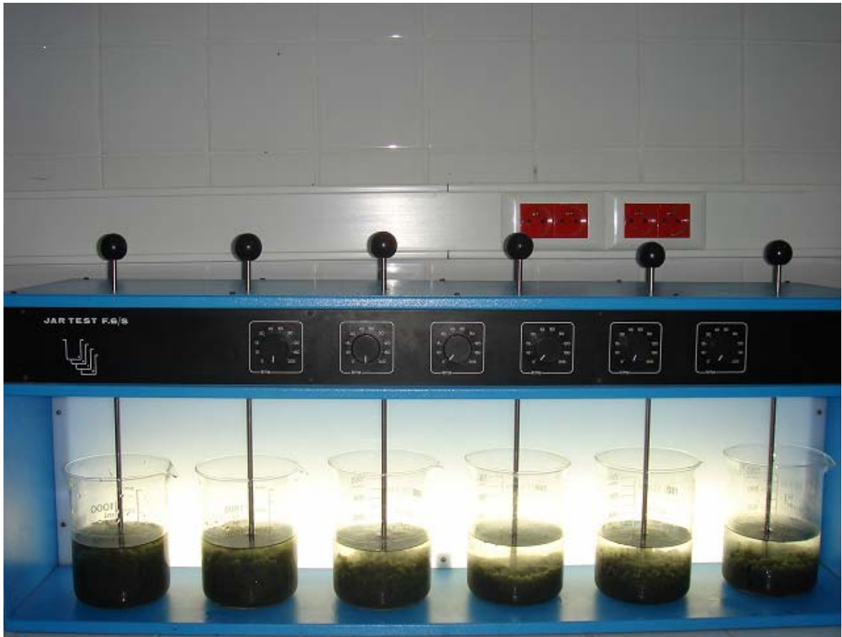
Figure 3.1. Jar test apparatus used in the experiments
